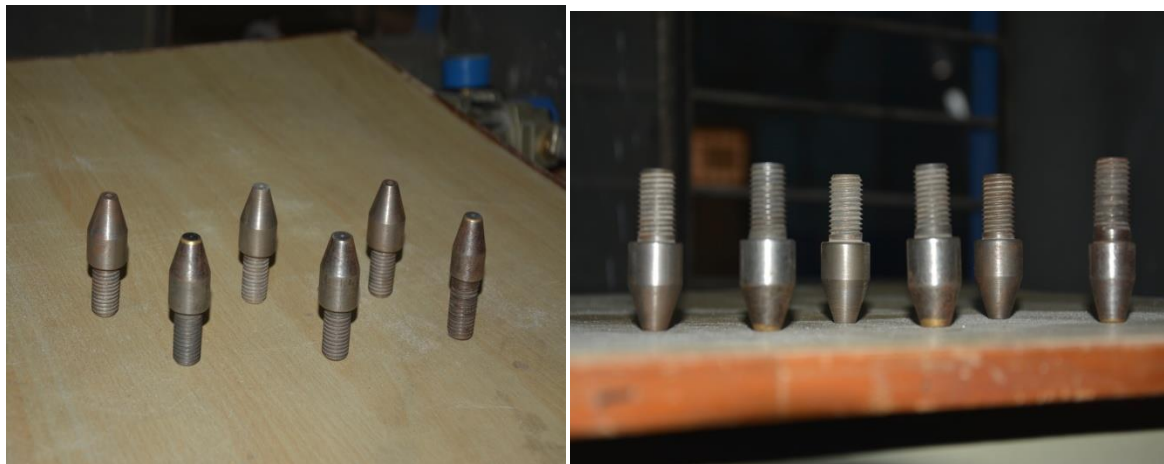
Fig.1 shows the different sizes of diameter of the Abrasive jet nozzle
