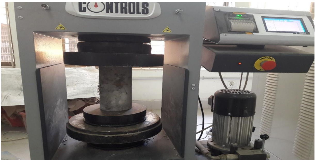
Fig.2. Compression testing machine
