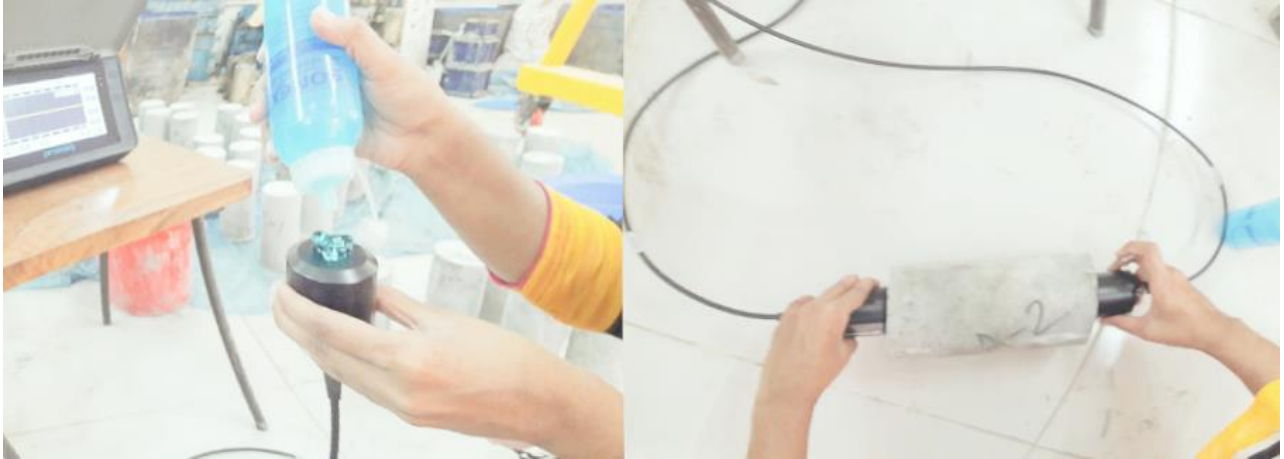
Fig.3: Ultrasonic Pulse Velocity Machine
