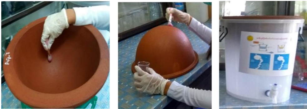
Fig. 1. SiAg Coating in ceramic water filter
