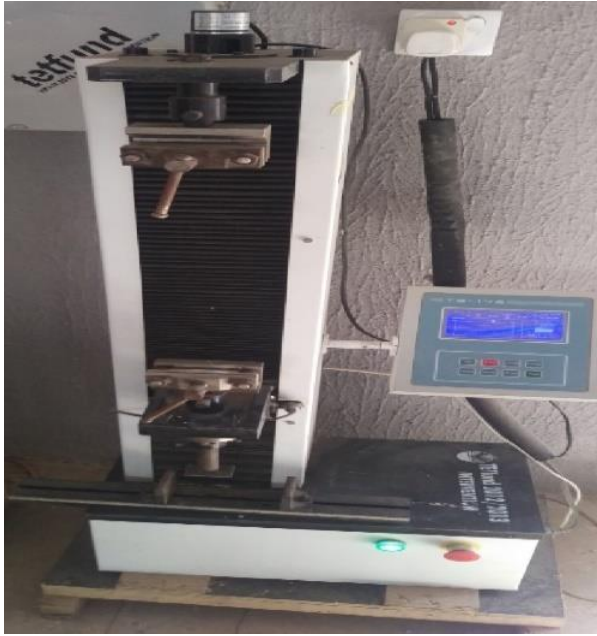
Figure 2: THE MARXTEST (TS 176). UTM machine.
